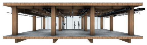
CLT / Concrete Composite System
